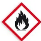
GHS02 and one of the hazard statements H224, H241 and H242 Flame
